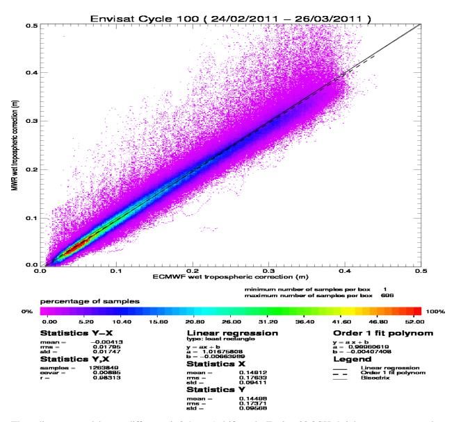
The radiometer-model mean difference is 0.4 cm. A drift on the Envisat 23.8GHz brightness temperature has been detected and has to be monitored on the long term. Note that the neural algorithm is now implemented on Envisat.
