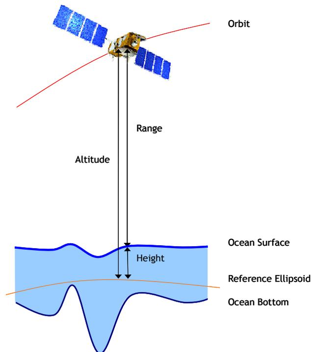
Figure 1 : Altimetric distances - Altitude, Range and Height
