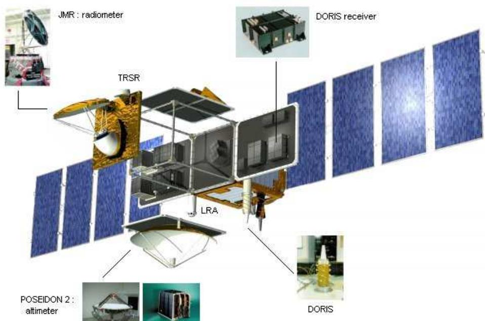
Figure 2 : Main components of the Jason-1 satellite
