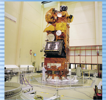
The ENVISAT satellite will carry a payload of several instruments including an altimeter that will be used for a mission complementary to that of Jason-1.
