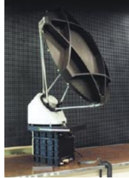
The radiometer, shown here with its antenna, is used to make precise measurements of the water vapor content of the troposphere and provide data to correct the radar altimeter measurements.
