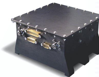
The GPS receiver, which receives up to 12 GPS satellites simultaneously, works with the DORIS system to calculate the satellite's trajectory.
