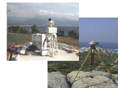
CNES, together with CERGA and IGN, have set up sea level and geodetic stations at Senetosa in Corsica to verify and calibrate Jason-1 altimetric measurements. The ultramobile laser station developed by OCA, CNES, IGN and INSU will support this campaign.
