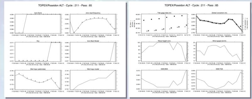
Figure 1b. Altimetric corrections for cycle 211.
