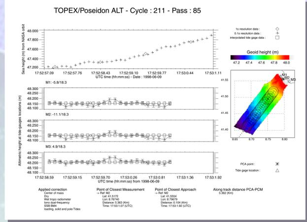
Figure 1a. Calibration process for cycle 211.
