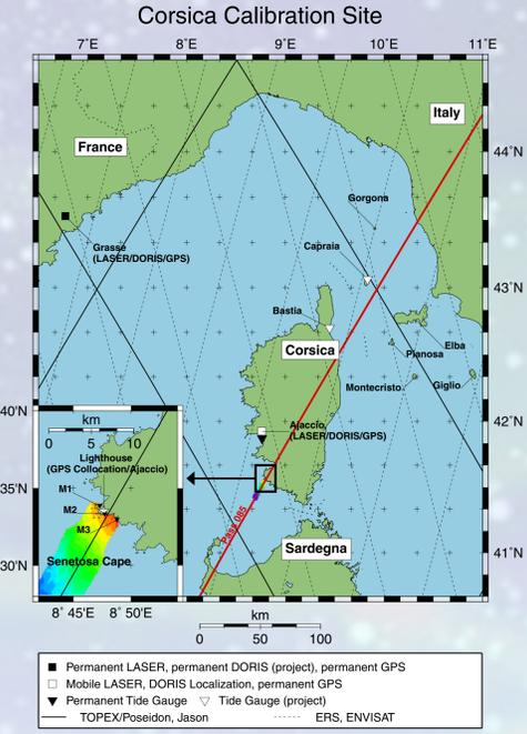
Plate 1. Configuration of the Corsica site. Contour map represents the geoid heights determined from Catamaran GPS measurements.
