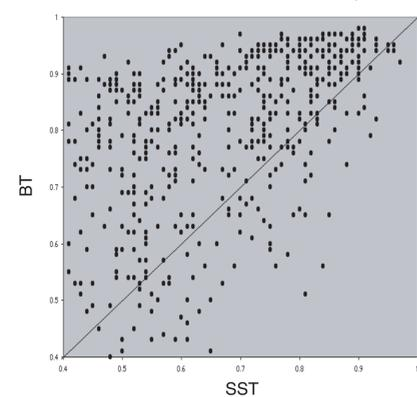
The maximum correlation coefficients from the BT fields were consistently higher than the those from the SST fields computed for 5 image pairs from the East Australian region (above), suggesting that BT fields provide a more reliable MCC velocity than SST. The lower correlation coefficients from the SST fields are hypothesized to be due to the introduction of noise through the differencing of radiometer channels in the algorithm used to derive SST.
