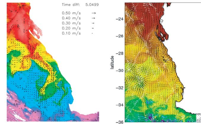
OIs were used to map MCC velocities (left panel) and altimeter-derived velocities (right panel) in the East Australian Current. As with the western Australia surface currents the features in the MCC current field are not identical with the geostrophic surface currents computed from the altimeter data. This is in part due to the higher spatial resolution provided by the infrared SST images which resolve the smaller scale current structures of the coastal region.
