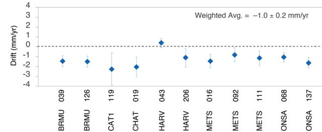
With the exception of the direct overhead pass at Harvest, all station/pass pairs yield a negative drift. The ensemble mean is  $-1.0 \pm 0.2$  mm/yr. Concluding this is due to the TMR requires a careful consideration of systematic GPS-related errors. Of particular concern are long-term changes in the abundance of low-elevation data. The following plot shows that the Harvest GPS site has experienced a slow degradation in the numbers of satellites tracked at low elevations:
