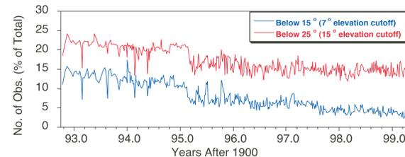
In contrast, the GPS station at Onsala has an extremely stable history of low-elevation tracking:
