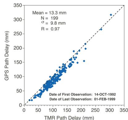
The close agreement between the TMR- and GPS-based PD estimates hints at the possibility of using time series of the differences for detecting subtle drifts in the radiometer. Provided in the following schematic are drift estimates (TMR–GPS) for the 11 station/pass pairs considered in the study:
