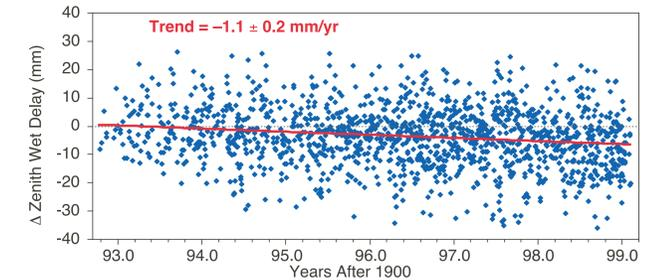
A downward trend, consistent with the TMR measuring PD shorter in time, is seen in the plot. The drift—also seen in comparisons with data from radiosondes and other radiometers—is attributed to hardware changes in the 18-GHz channel from 10/92 to 12/96 [Keihm et al., 1999]. The following figure shows the TMR–GPS time series after correcting for the effects of the 18 GHz drift. To isolate the impact of the correction, the time series is divided into two segments—before and after 12/31/96.
