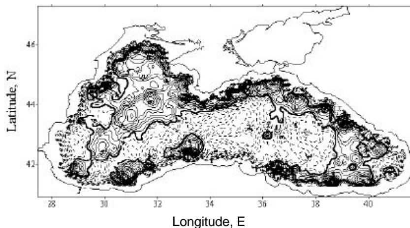
Root mean square sea level deviation based on ERS-1 altimetry. Values smaller than 4 cm are denoted by a dotted line; contour intervals are 0.25 cm. Korotaev, G.K., Saenko, O.A., Koblinsky, C.J., "Satellite Observations of the Black Sea Level", submitted to Journal of Geophysical Research.
