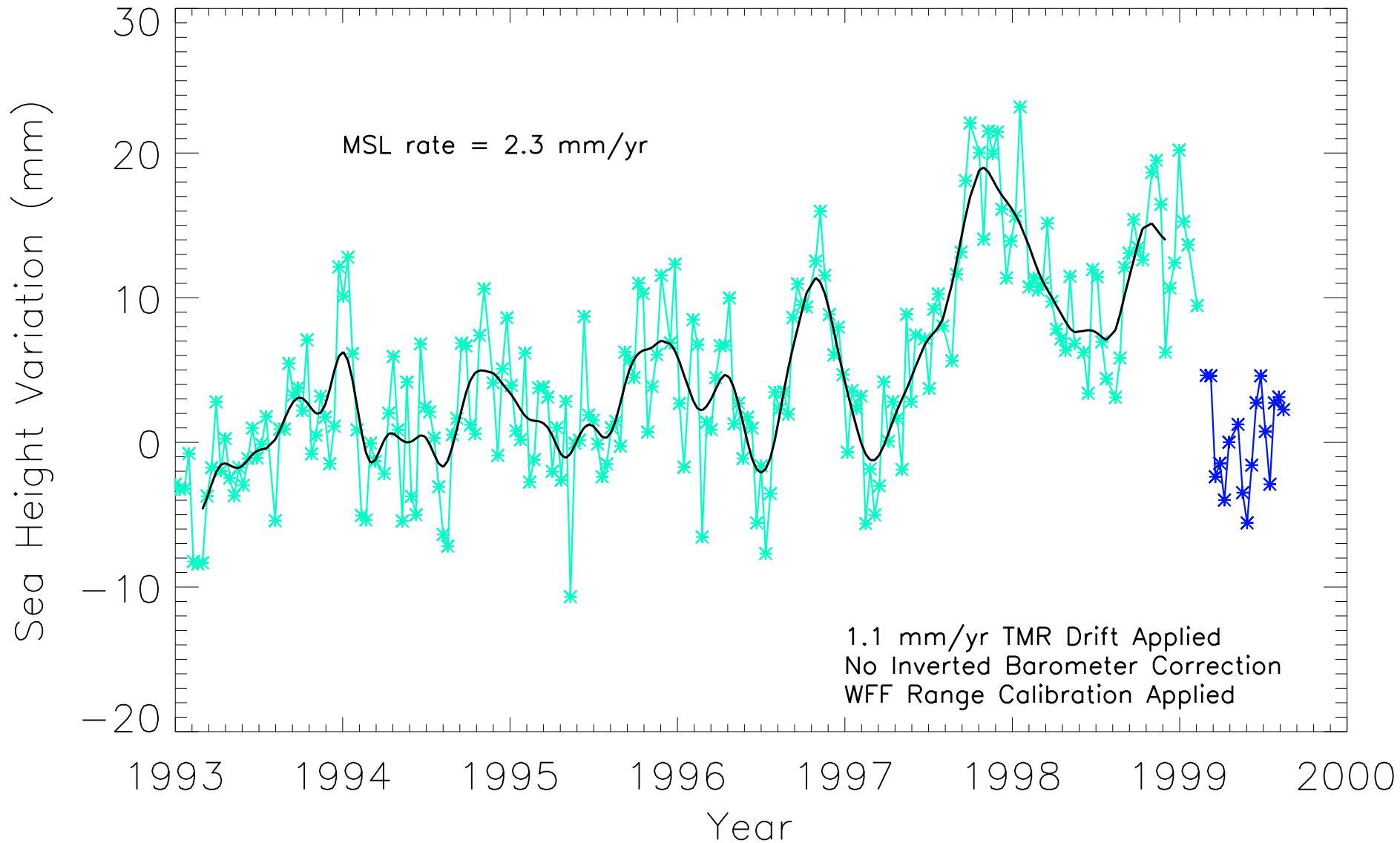
Global mean sea level variations are computed from TOPEX/POSEIDON altimetry for cycles 10 - 254. Each asterisk represents a 10 day estimate of the global mean sea level variation with respect to a 1993-1996 average. The solid black line is a 60-day Hanning filter. The dark blue points identify the transition to ALT B that is currently being validated.
