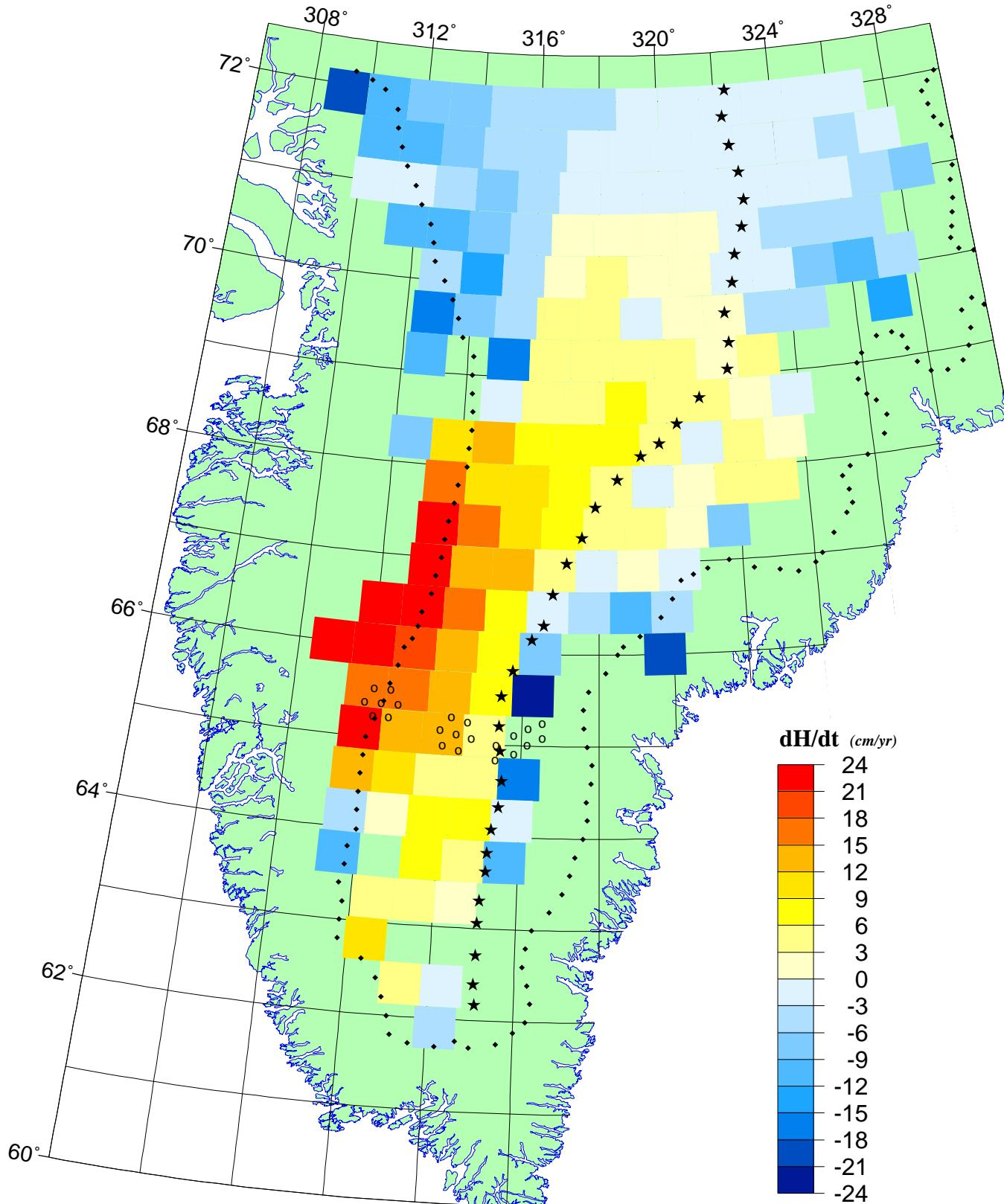
Elevation changes in the Greenland ice sheet are measured from the Geosat GM, ERM and Seasat altimetry. Courtesy of Davis, C.H., C.A. Kluever, B.J. Haines, C. Perez, and Y.T. Toon (1999), "Improved elevation change measurement of the Greenland ice sheet from satellite radar altimetry", IEEE Transactions on Geoscience and Remote Sensing, in press.
