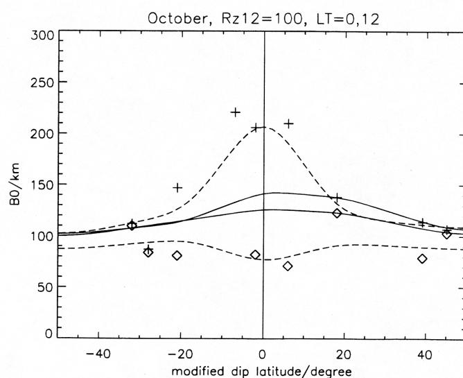
The above figures show the bottomside thickness  $B_0$  plotted against modified dip latitude for high solar activity ( $Rz12=100$ ) for the spring and fall equinox.  $B_0$  determines the IRI electron density profile below the F peak and thus about 35 to 50 % of the Total Electron Content (TEC). The ionospheric correction of altimeter measurements is directly proportional to the ionospheric Total Electron Content (TEC) between the satellite and the ground.
