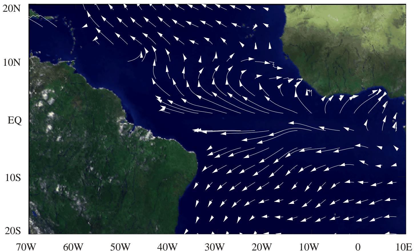
The top image is a mean ocean surface velocity obtained by ship drift data (Richardson and Walsh [1986]). The bottom image shows a similar ocean surface velocity field derived from TOPEX/POSEIDON altimeter data and SSMI wind data.
