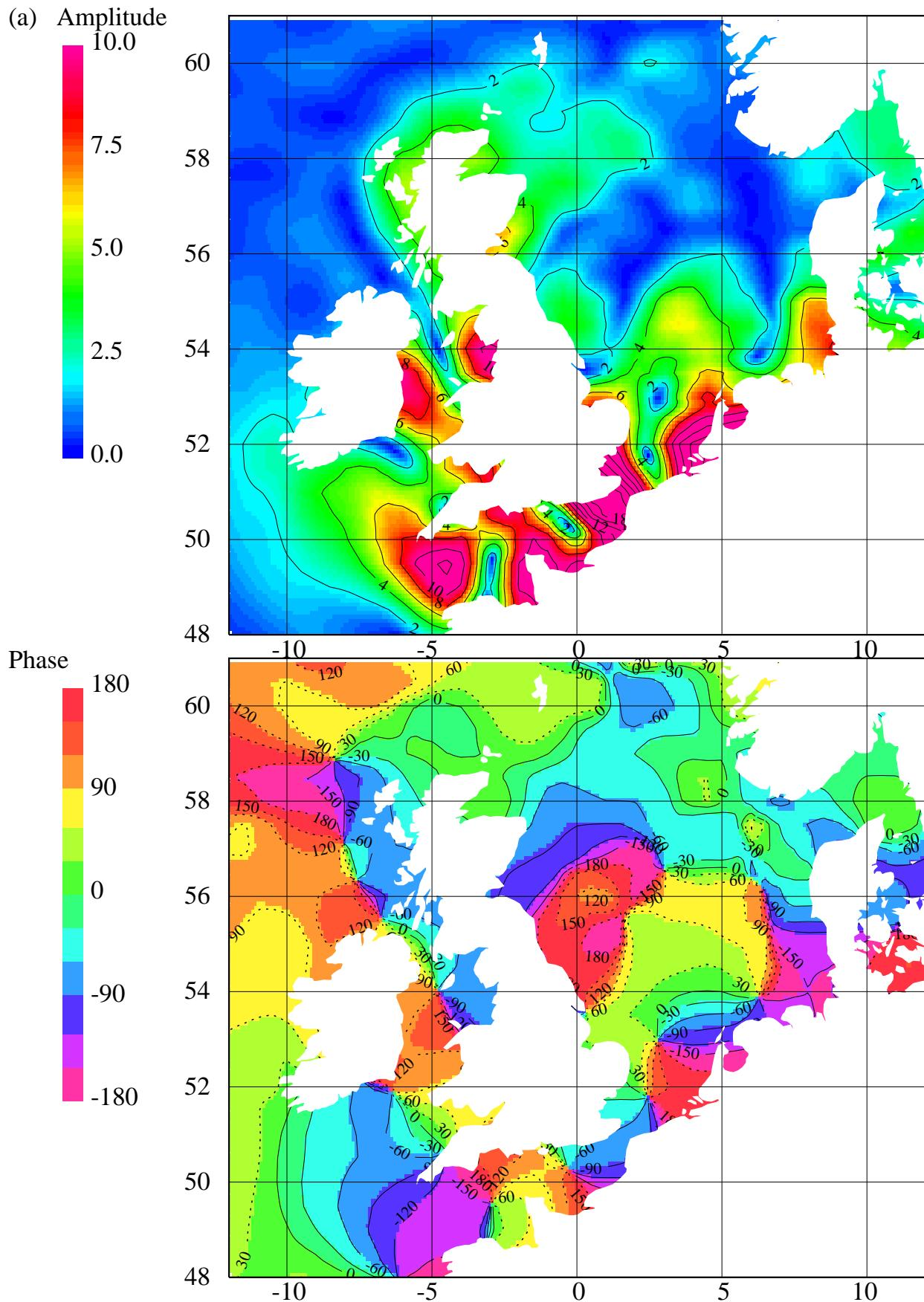
The shallow water M4 constituent in the northwest European shelf region derived from T/P data. Amplitudes are in centimeters, and phases are in degrees with respect to Greenwich. Note the ability of the T/P data to resolve high frequency shallow water tides. Reference: O.B. Andersen, Shallow water tides in the northwest European shelf region from TOPEX/POSEIDON altimetry, Journal of Geophysical Research, Vol 104, C4, April 15, 1999.
