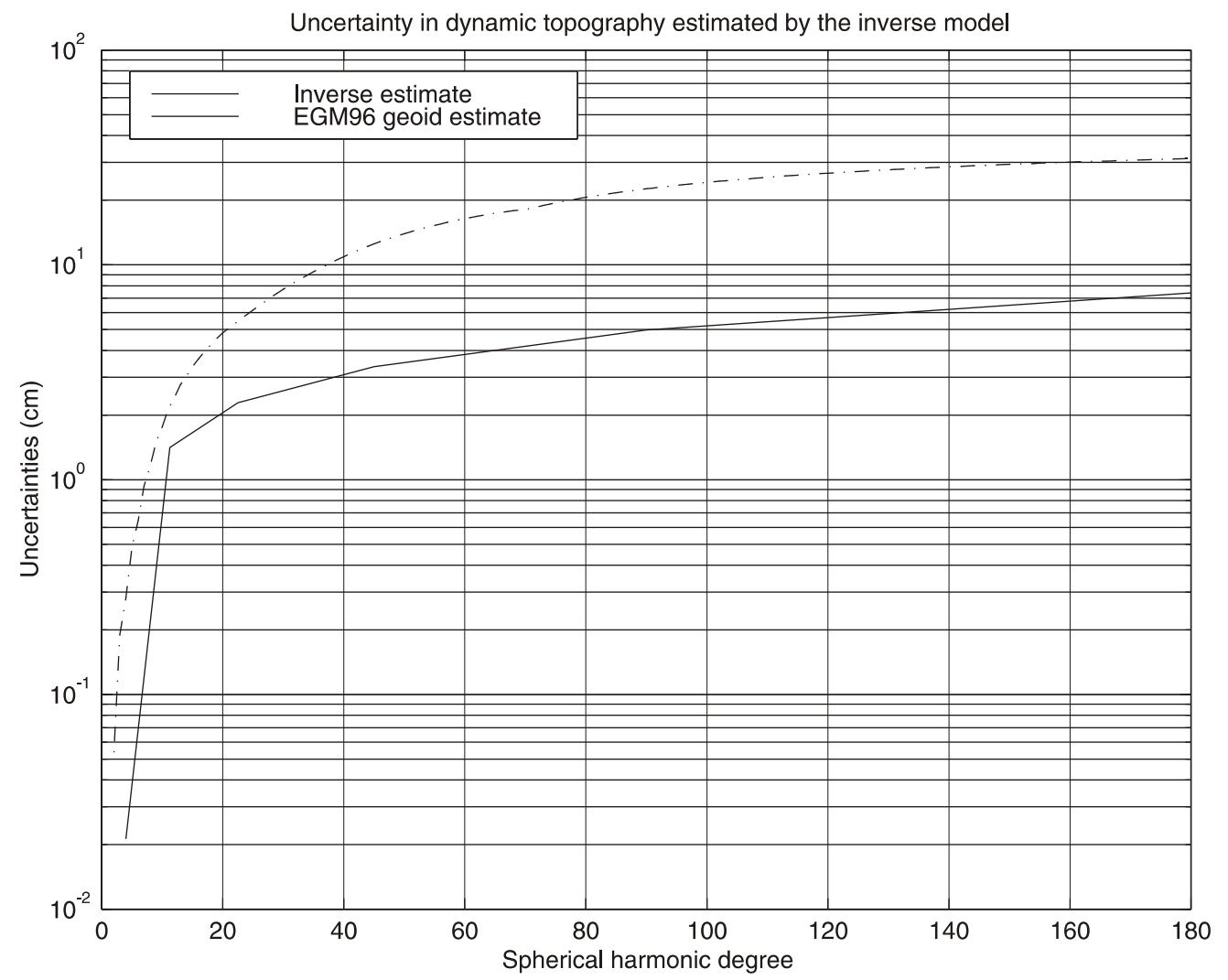
Figure 3: Uncertainty in the inverse estimate of mean dynamic topography as a function of spatial scale (presented in terms of spherical harmonic degree).
