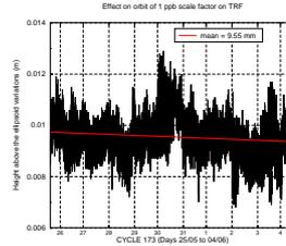
Similar procedure was used with a scale factor transformation applied to a Terrestrial Reference Frame (1 ppb). Effect on orbit seems to be very significant if we consider this case with a mean value about 1 cm and a standard deviation about 1 mm.
