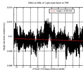
In case of scale factor the orbit error and the mean sea level evolution coming from a scale factor of 1 ppb applied to the terrestrial reference frame is exactly the same : 10 mm for 1 ppb. This similarity explains itself because the orbit will be identically transformed wherever we look around the earth, so results on Mean SEA Level (MSL) are independant from the ocean dissymetry.
