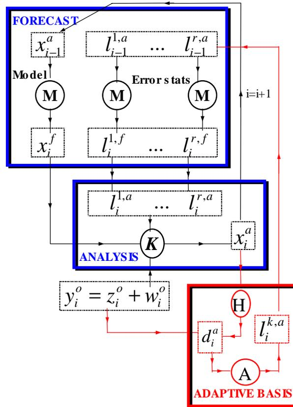
*Schematic representation of the sequential SEEK algorithm*
