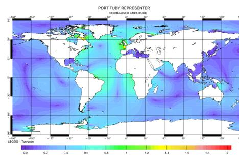
Figure 5 : Representer associated to a coastal tide gauge ( $M_2$  normalised amplitude)
