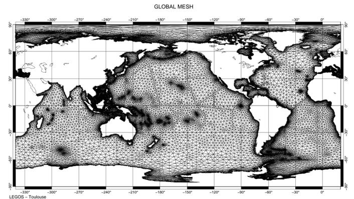
Figure 1 : Global finite element mesh used to compute FESs
