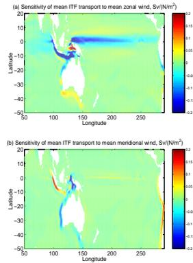
Fig. 1 Sensitivity of annual mean ITF transport to unit positive perturbation in annual mean zonal (a) & meridional (b) wind stress. Positive values indicate enhanced ITF.
