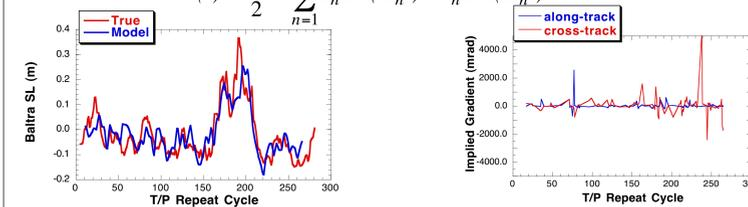
Real sea level variability and model based on SOI and PDOI
