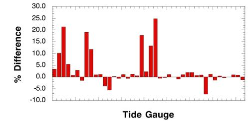
This shows the % difference change in the tide gauge residuals, where  $\sigma$  is std. dev. of sea level residual (T/P - tide gauge), and + values indicate  $\sigma_{7yr} > \sigma_{4yr}$
