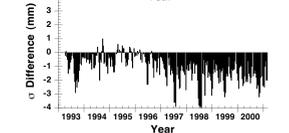
Difference in global standard deviation of TOPEX sea level anomalies relative to MSS models. Previously, the 7yr model only decreased  $\sigma$  for a few cycles. Now,  $\sigma$  is decreased for most cycles.
