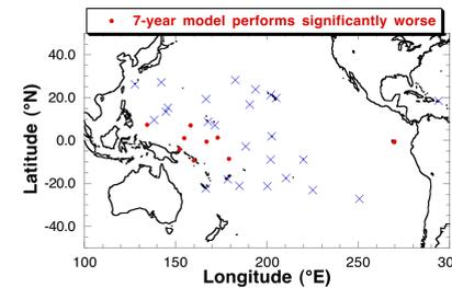
Locations of tide gauges. Red dots indicate where 7-yr MSS produces worse residuals than 4-yr MSS
