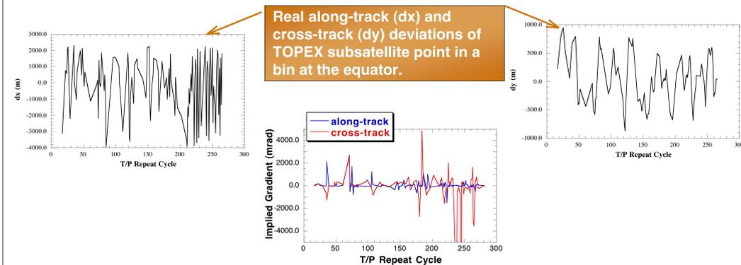
False gradients implied by real variability (found by dividing real  $\Delta\eta$  by dx or dy). In order to estimate true gradients in the presence of this, the averages must be nearly zero. In fact, they are about 60  $\mu\text{rad}$  for along-track and 144  $\mu\text{rad}$  for the cross-track. For comparison, the estimates from the 4-year model for the absolute gradients are -27 and 7  $\mu\text{rad}$ , respectively, for this bin.
