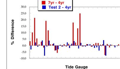
% difference change in the tide gauge residuals for the old 7yr model (red) and the new 7yr model (blue). Now, no comparison is significantly worse when 7 years of data are used than when 4 years are used.
