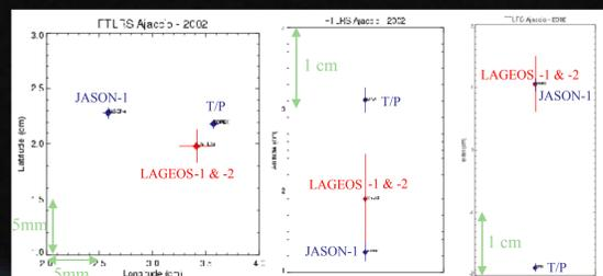
The FTLRS has been settled at Ajaccio geodetic site (7848) since from January to September 2002. Its tracking location allows quasi-zenithal observations of Senetosa calibration pass N°85. Very accurate short-arc orbits can then be computed and used in the altimeter calibration process. Moreover, the FTLRS and also the Grasse station have the capability to switch from Jason-1 to T/P during passes.
