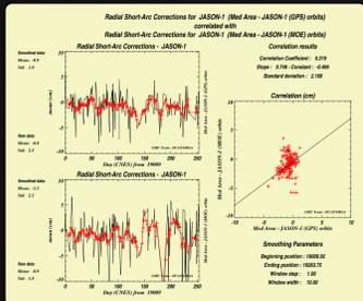
In this section MOE using GPS or DORIS have been compared. The GPS ones seems to have a better stability in the radial component (13 mm and 19 mm for the standard deviation respectively above the Mediterranean and the USA areas).
