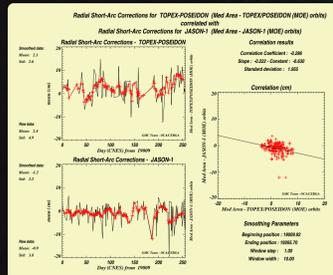
The radial precision of Jason-1 MOE has been improved in comparison to T/P ones. Stability is near the level of T/P POE while for T/P MOE its stability remain higher. No correlation can be evidenced between both MOE.
