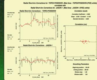
Jason-1 POE orbits has been studied from cycle 1 to 20 and correlated with T/P POE on the corresponding cycles. The radial component of Jason-1 orbits seems to be more stable. Moreover, the radial precision has been improved by 12 mm over the Mediterranean area while this improvement is just 1 mm over the USA area.
