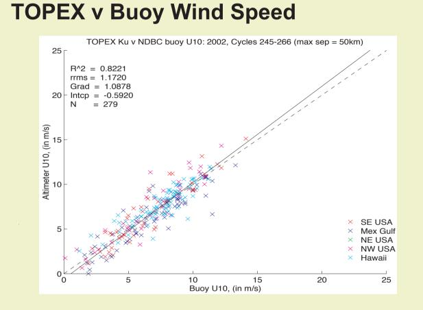
**Calibration correction:** U10(cor) = 0.8375 U10(T) + 1.1720 conf limits 0.7370 - 0.9380 0.8692 - 2.4035 resid. rms=1.1720m/s
