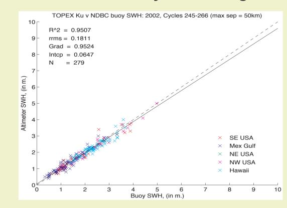
**Ku Calibration correction:** □ Hs(cor) = 1.0520 Hs(T) - 0.067495% conf limits □ 1.0233 - 1.0806 -0.1227 - -0.0121 resid. rms=0.1811m
