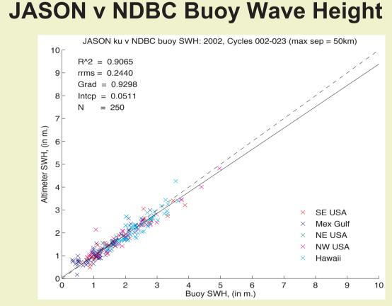
**Ku band Calibration correction:** Hs(cor) = 1.0472Hs(JKu) - 0.0137resid. rms=0.2440m 95% conf limits 0.9954-1.0991 -0.1116 - +0.0842
