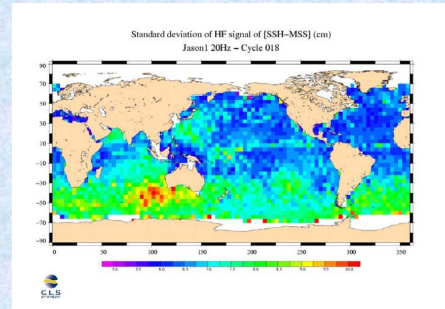
The above figure shows the geographical pattern of the HF signal. It is strongly correlated to SWH (bottom figure), but wet areas also appear (rain situations).
