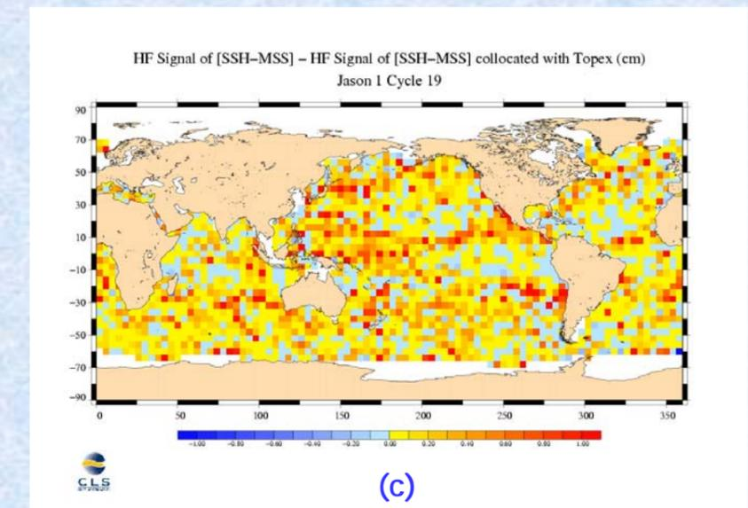
Yellow/red boxes on figures (b) and (c) mean reduction of Jason-1 HF signal after collocation with Poseidon-1 or Topex. Poseidon-1 and Jason (Poseidon-2) data editing are consistent, but collocating Jason-1 with Topex leads to significant HF signal reduction, particularly on wet areas. Note that in these rainy areas a significant amount of Topex data is edited due to the waveform off-nadir angle parameter (not computed).
