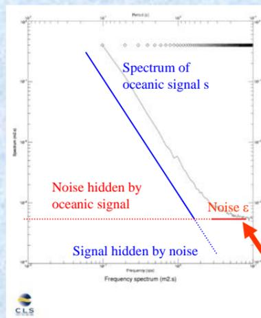
A plateau on a power spectrum can be the signature of a white noise. The STD of its distribution can be obtained by :
