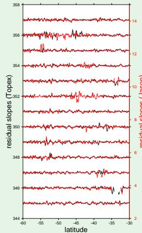
Time series for track 'a003' in the Southern Ocean show that TOPEX and JASON measurements are roughly in agreement although both instruments show signs of anomalous events. Data processing methodology adapted from Yale et al. [1995].
