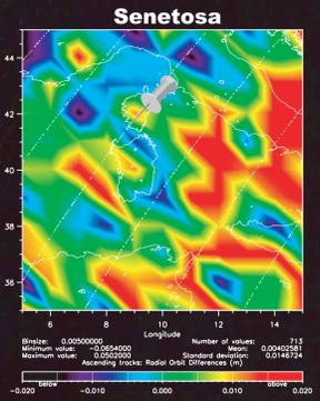
Radial orbit accuracy shows a very good consistency between POE, GPS RD and Short-Arc. In this area the Geographically Correlated Error is negligible (below 2 mm). However, radial orbit differences from all the studied orbits reveal a change in the MOE behavior before and after the validation period. This is can be due to the fact that the Cal/Val phase was a period used to tune the orbit determination process.
