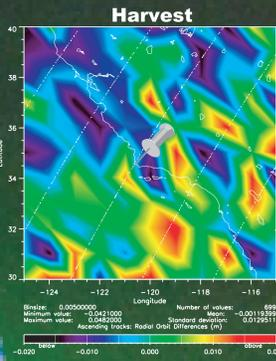
Radial orbit accuracy shows a very good consistency between POE, GPS RD (with GRACE) and Short-Arc. These three kinds of orbit reveal clearly that MOE is biased by about 8 mm. However, GPS RD based on JGM3 is closer to MOE and then exhibit a Geographically Correlated Error at the level of 6 mm.
