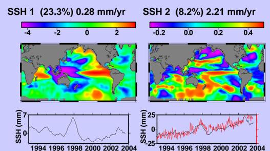
Figure 12. Leading sea level EOFs for T/P and Jason. Mode 2 shows significant correlation with global mean sea level (red). Seasonal terms have been removed.
