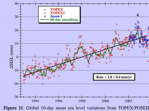
Figure 11. Global 10-day mean sea level variations from TOPEX/POSEIDON and Jason-1. No tide gauge calibration has been applied. No inverted barometer correction has been applied to the time series.
