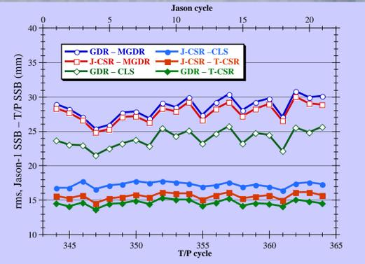
Figure 2. Root mean square of the difference in the global mean sea state bias corrections from T/P and Jason-1 during the calibration phase.
