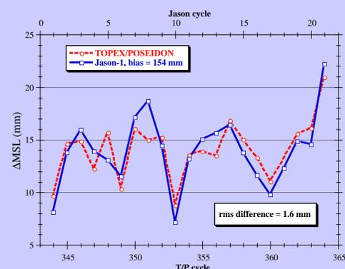
Figure 5. Ten-day global mean sea level estimates from T/P and Jason-1 during the calibration phase. A 154 mm bias has been removed from Jason-1. The zero level of the time series is the mean sea level during the original T/P mission.
