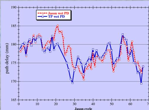
Figure 1. Wet troposphere path delay from Jason-1 and T/P. The TOPEX path delays have been corrected for yaw-related bias and a constant bias.
