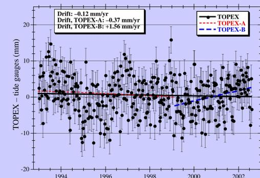
Figure 7. The present estimate of the TOPEX drift computed from the global tide gauge analysis. The solid dots and error bars are the estimates that are computed independently for each cycle of the TOPEX data, and the solid line is the result of fitting a linear trend to the data.
