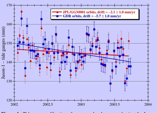
Figure 4. Tide gauge calibration of mean sea level computed using the Jason GDR orbits and JPL orbits.
