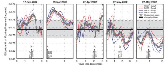
Results of the GPS solutions, relative to the mooring-derived SSH, for the five GPS buoy deployments. The solid horizontal line is the mean over all deployments and the heavy grey lines show the mean of all four solutions (2 x GPS buoys vs 2 x GPS ground stations) for each deployment. The solid and dashed coloured lines show the four separate solutions.
