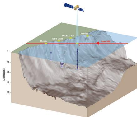
During the "Formation Flight" period (January to August, 2002) when Jason-1 and TOPEX/Poseidon were flying over the same ground track with Jason-1 approximately 70 seconds ahead of TOPEX/Poseidon we deployed an array of oceanographic instruments off Burnie.
