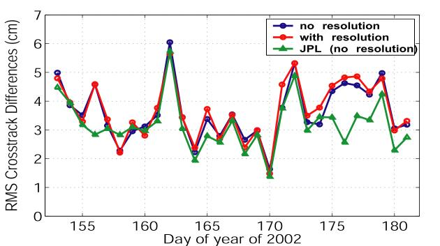
The orbit agreement with SLR/DORIS derived solutions are within 2 cm (except for DOY 155) in the radial component. On an average, the crosstrack and alongtrack components of the orbit agree to 3.8 cm and 4.1 cm respectively. Ambiguity resolution has mm-level effect on Jason-1 orbit solutions. Thus, the changes are not eminent in the plots.
