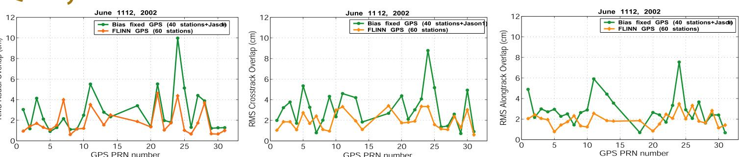
The estimated GPS orbits in the POD processing are compared to JPL FLINN precise (final) GPS solutions. The orbit overlap statistics for period June 11 and 12, 2002 show that the estimated GPS orbit quality is within 6 cm in all directions except for GPS PRN 24. The statistics for all other days are of similar quality.
