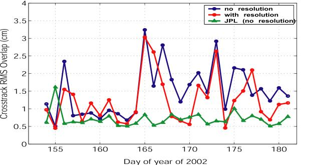
The statistics are obtained from a 4-hour orbit overlap period (with respect to the day after) between 2 consecutive days. The mean improvement in the radial component is 1.4 mm after resolving phase ambiguities. The crosstrack and alongtrack components show an average improvement of 2.5 mm and 3.9 mm respectively. The POD processing for Jason-1 is similar to that of JPL except
