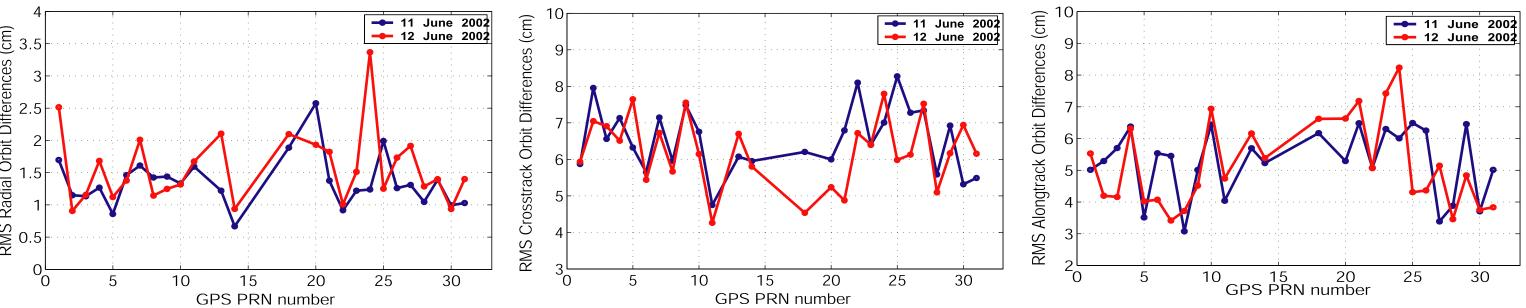
The above 3 plots are RMS orbit differences between the estimated GPS bias fixed orbits and the FLINN GPS precise solutions. The mean orbit agreement for both days is approximately 1.5 cm, 6.4 cm and 5.3 cm in the radial, crosstrack and alongtrack respectively.
