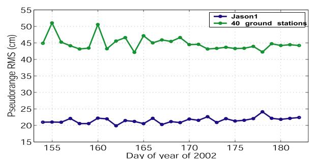
The orbit fit for Jason-1 has an average RMS of 5.6 mm and 21.5 cm for the pseudorange and carrier phase respectively over 29 days. The ground station measurements show an average RMS of 6.4 mm for the phase and 44.9 cm for the pseudorange.
