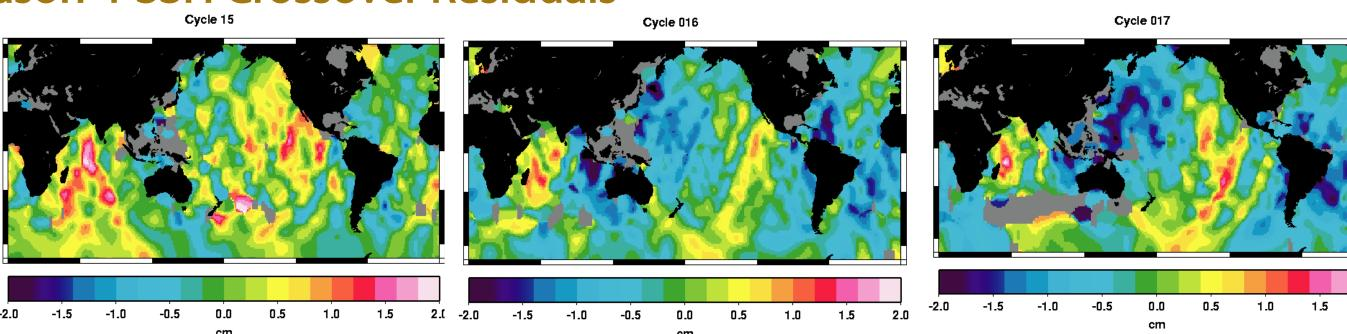
The above sea surface height (SSH) residual representations show the magnitude of the ocean signals that are removed after ambiguity resolution.
