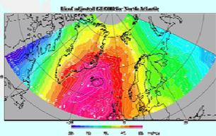
Figure 2. The final FFT-GRACE geoid of the North Atlantic region. The geoid accuracy should be better than 10 cm.
