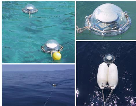
Fig. 2: GPS equipped buoys deployed in coastal region (upper pictures) and offshore (lower pictures), where the pulled buoy is attached to a floating construction to maintain buoyancy. The shell of the buoys is fabricated from microwave-transparent polycarbonate, so they can be waterproofed sealed containing the receiver (NovAtel DL-4), antenna and battery.
