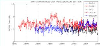
Times series (left figure) of 10-day averages of SWH over the global ocean show significant differences among the altimeters (first figure on the right). Using the swh altimeter data correction (Queffeuou 2004) allows to reduce the differences to less than about 15 cm (second figure on the right). Could this residual be reduced, with improved corrections, or does it result from the different time and geographical samples of the global ocean by the various altimeters?
