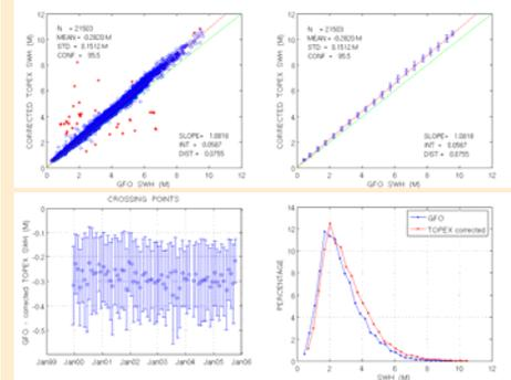
SWH measurements from GFO (raw) and TOPEX (corrected) at crossing points are strongly correlated. Mean value of differences is about 28 cm, with a 15 cm standard deviation. The slope (1.0818) and intercept (0.0587) of the orthogonal regression line can be used to correct the GFO SWH data.
