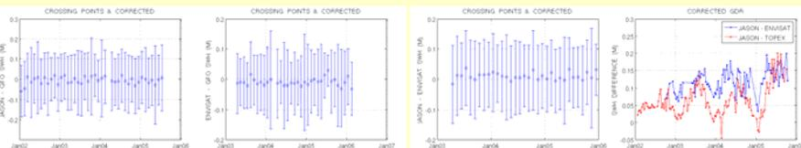
Monthly mean SWH differences between JASON and ENVISAT, at crossing points, are close to zero (left). Nevertheless, the 10-day mean value differences for global ocean (right) are larger and fluctuate due to different time and geographical samplings and to possible remaining differences at high SWH.
