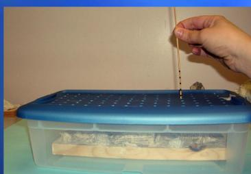
Sampling the topography with bamboo “altimeters.”
