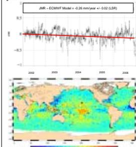
Figure 4: Global (top) and local (bottom) slope estimation of the difference between radiometer and model wet troposphere correction.
