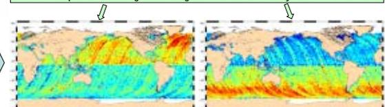
Figure B4: SLA differences using new orbits (GFSC200 for J1 and T/P) and new ranges for ascending (left) and descending (right) passes [cm]
