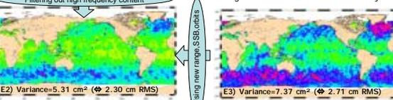
Fig. E1: Variance of SLA differences [cm<sup>2</sup>] using new orbits and new ranges; fig. E2 : same fig. E1 after filtering out SLA signal smaller than 50 km; fig. E3: same fig. E2 using old orbits and old ranges.
