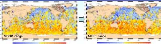
Fig. B3: SSH differences at TOPEX crossovers with the MGDR Range (left) and MLE5 range (right). TOPEX MLE5 range increases the hemispheric ascending/descending differences
