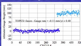
TOPEX and Jason-1 sea surface height variations are compared to tide gauge variations from 64 sites. Altimeter SSH values are based on GSFC ITRF2005 (GGM02c) orbits, and most recent recalibrated TMR and JMR wet tropospheric range corrections. After adjustment of the decimeter level instrument bias computed from Jason-TOPEX collinear differences during the verification phase, the total residual drift equals -0.11 mm/yr.
