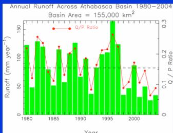
Model-derived runoff was 164 mm/year in 1996, more than double the 25 year mean. Above average runoff occurred for 5 years from 1993-1997. Q/P ratio was highest in 1997. It looks like snowfall/melt forced the anomaly in 1996 and 1997?
