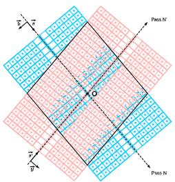
Fig 3 : WSA crossover diamond. Two measurements on the same location can be used to estimate the roll-induced SSH signal
