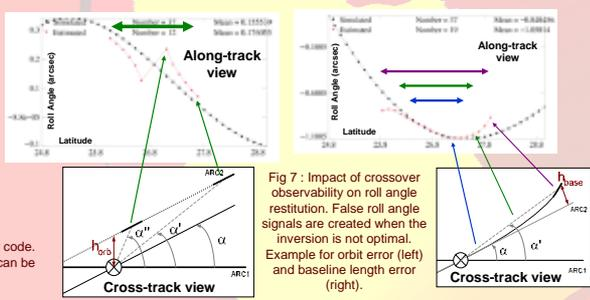
Fig 7 : Impact of crossover observability on roll angle restitution. False roll angle signals are created when the inversion is not optimal. Example for orbit error (left) and baseline length error (right).
