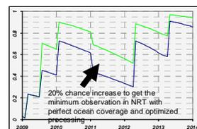
Fig 6 : Probability to have the minimum NRT observability with opportunistic ocean data from CryoSat (blue) and with perfect ocean coverage and improved geophysical corrections (green).
