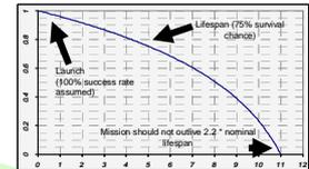
Fig 1 : Probability function used for an altimeter with a 5 year lifespan
