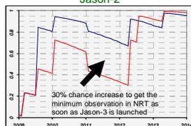
Fig 7 : Probability to have the minimum NRT observability with a Jason-3 launch in mid 2012 (red) or in mid 2009 (blue).
