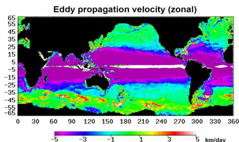
**Features to note:** equatorial eastward high-speed zone (up to 70 km/day), subtropical westward high-speed zone (up to 25 km/day), high speed zone in barotropic gyres (south of the Gulf Stream, Argentine basin), eastward velocity in the Gulf Stream, ACC.
