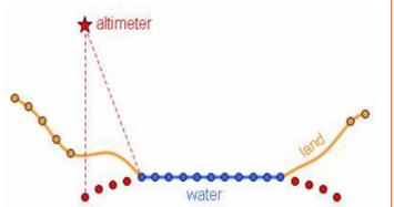
Figure 2b: DEM sampling along the orbit path. Extension of areas of interest (water) and slant view correction.
