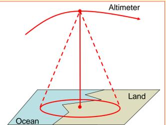
Figure 2a: DEM sampling along the orbit path. As oceans have a higher priority than lands, the nadir point is assigned to an ocean point.
