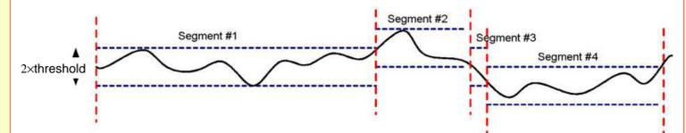
**Incremental coding**: For memory size optimization, successive points with higher altitude variations are coded as follows: Altitude of the first point (2 bytes), then altitude increments (1 byte each).
