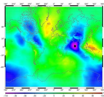
Figure 3: Elevations of the Eigen geoid truncated at order 78 wrt WGS 84 ellipsoid.
