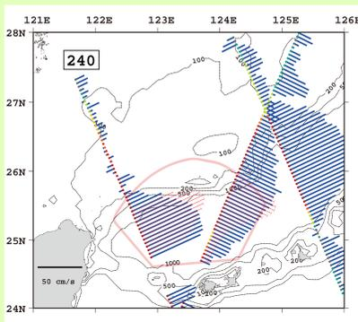
Fig. 2-4: 3.5-year mean velocity component normal to the track. The HF velocity is also plotted with red arrows.
