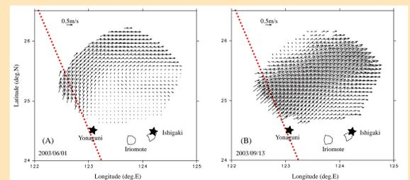
Fig. 4-2: The surface geostrophic velocity estimated from the HF data on 1/June/2003 (A) and 13/Sept/2003 (B).
