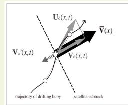
Fig. 2-1: Schematic diagram for estimation of mean component  $\bar{V}(x)$  from drifter velocity  $U_d$  and altimetry geostrophic anomaly component  $V_a'$ .
