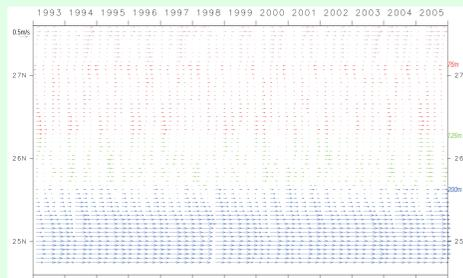
Fig. 3-1: Time series of 90-day averaged velocity component normal to the track 240. Arrows are colored in blue, green, red and pink, if the depth of the points is deeper than 200m, 125-200m, 75-125m and shallower than 75m, respectively. A rightward arrow indicates northeastward flow.
