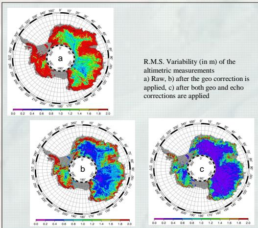
R.M.S. Variability (in m) of the altimetric measurements
