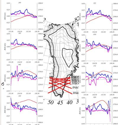
The 8 tracks studied are displayed over the Greenland topography on the top plate. The corresponding surface height trends as measured by Topex are displayed on the eight other plates from top to bottom as from north to south. The trends are drawn in pink for Ku Band and in blue for C Band. The geoidic surface height is also displayed in red.
