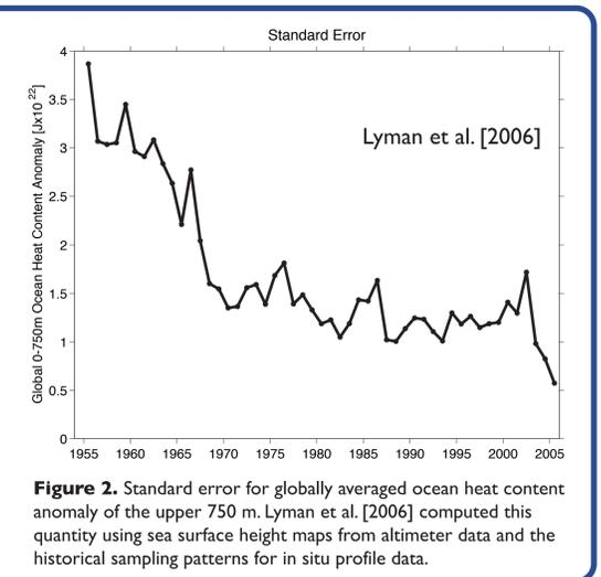
Figure 2. Standard error for globally averaged ocean heat content anomaly of the upper 750 m. Lyman et al. [2006] computed this quantity using sea surface height maps from altimeter data and the historical sampling patterns for in situ profile data.
