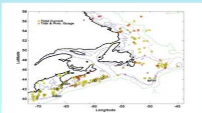
**Figure 2** Observations for comparison with the model were taken primarily from the southern portion of the domain. Data were used from coastal tidal gauges, bottom pressure gauges (Han et al., 1996) and current meters (Drozdzowski et al., 2002). There are 52 locations for elevation and 334 sites/positions for currents.
