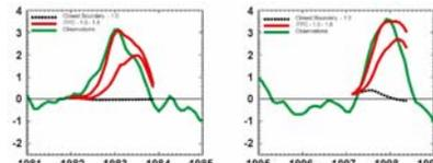
Figure3b-c: NINO3 SST indices simulated in coupled contexts without ITF (black) or with ITF values prescribed at the western boundary of the model (red). Green is Reynolds observed SSTs.
