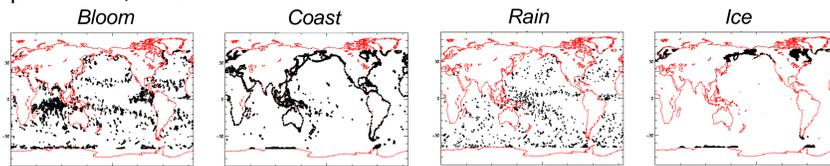
In these models, the classification result is presented as a graph called « **topological map** » where resembling categories (classes of altimetric waveform shapes) are close spatially. The results have shown that the **classes are labeled with more than 93% success** for the ocean, 100% for land surfaces, 88% for sea ice and 100% for coasts types.
