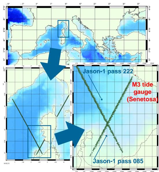
Fig.2: Jason-1 data available for passes 085 and 222 in the x-track SSH product for cycles 1 to 135
