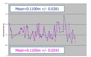
Fig.5: SSH absolute bias at M3 tide gauge, Jason-1 pass 085 (51 common exploitable cycles). Pink curve: no correction; blue curve: tides and ocean response to atmospheric forcing corrected
