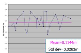
Fig.4: SSH absolute bias at M3 tide gauge, Jason-1 pass 222 (27 exploitable cycles).
