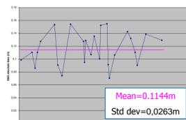
Fig.4: SSH absolute bias at M3 tide gauge, Jason-1 pass 222 (27 exploitable cycles).
