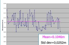
Fig.3: SSH absolute bias at M3 tide gauge, Jason-1 pass 085 (86 exploitable cycles).
