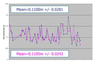
Fig.5: SSH absolute bias at M3 tide gauge, Jason-1 pass 085 (51 common exploitable cycles). Pink curve: no correction; blue curve: tides and ocean response to atmospheric forcing corrected
