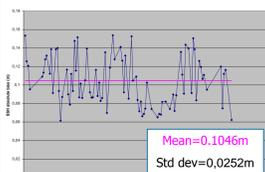
Fig.3: SSH absolute bias at M3 tide gauge, Jason-1 pass 085 (86 exploitable cycles).
