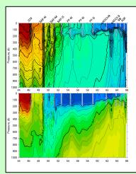
Potential temperature (top) and salinity (bottom) in the upper 1000 m along the WOCE/CLIVAR SR3 line at 140°E in November 2001. Each of the major ACC fronts is split into multiple filaments.
