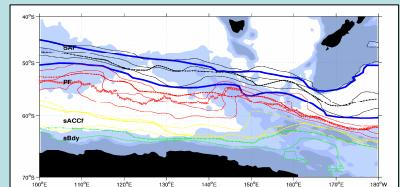
Comparison between Southern Ocean front positions mapped using SSH and positions reported by Belkin and Gordon (1996, thick blue line), Orsi et al. (1995, solid lines with open triangles) and Moore et al. (1999, solid lines with open triangles). The Southern Ocean fronts (except Belkin and Gordon) are color-coded: SAF – black, PF – red, sACCF – yellow, Bdy – green, SAZ/STF – blue. The bathymetry is shaded grey (the 4000, 3000, and 2500 m contours are shown).
