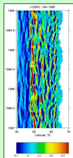
Meridional SSH gradient (m/100 km) at 130°E between 1994 and 1997. The ACC consists of multiple filaments that merge and diverge, but the jets also persist for many months.
