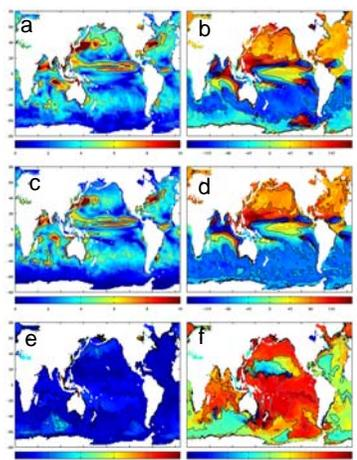
Figure 4: Annual cycle (amplitude in cm, and phase in deg) for the full sea level (a,b), thermosteric height (c,d), and bottom pressure (e,f). Phases are as in  $\cos(\omega t + \phi)$ .
