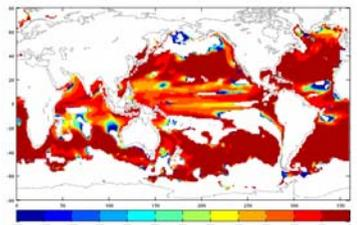
Figure 5: Depth to which it suffices to integrate the steric height in order to explain > 80% of the annual SSH signal. Blank areas are regions where bottom pressure is important.
