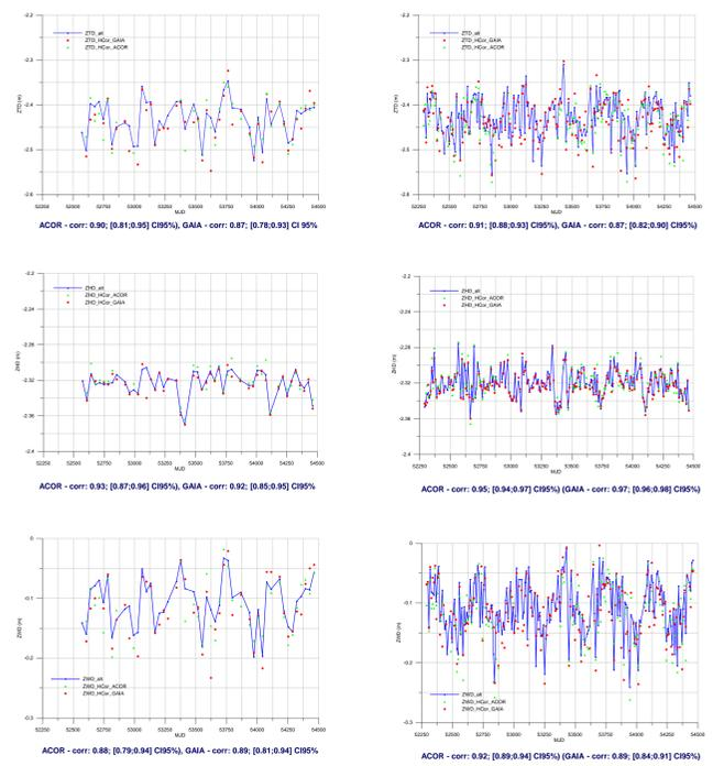
From left to right figures show UPorto GAMIT ZTD, ZHD and ZWD, before (in red) and after (in green) applying height correction for GAIA station (H=232 m), for the period 2002-2007.
