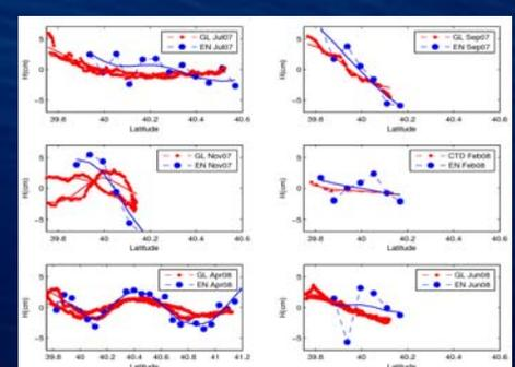
Raw (dashed-dotted) and filtered (continuous) glider and ENVISAT data. For the glider measurements, both sections (go and return) are displayed when available.
