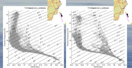
Glider TS diagrams for S1(left) and S2(right). Both TS have a branch of recent AW, while only S2 reveal the presence of old AW (higher salinity values).
