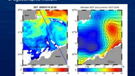
Left: SST image. Data provider: EUMETSAT. Right: ADT (cm) and geostrophic currents (cm/s) from real time altimetry merged maps. Data provider: AVISO.
