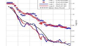
Fig. 8: Dynamic height at 2000db (blue and red dots) and at the isopycnal 27.86 (blue and red lines) and Rio05 (dashed black line)
