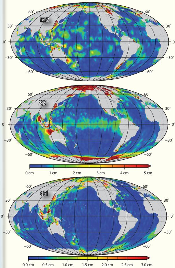
Fig. 1: Residual amplitudes for M2, S2 and O1 constituents
