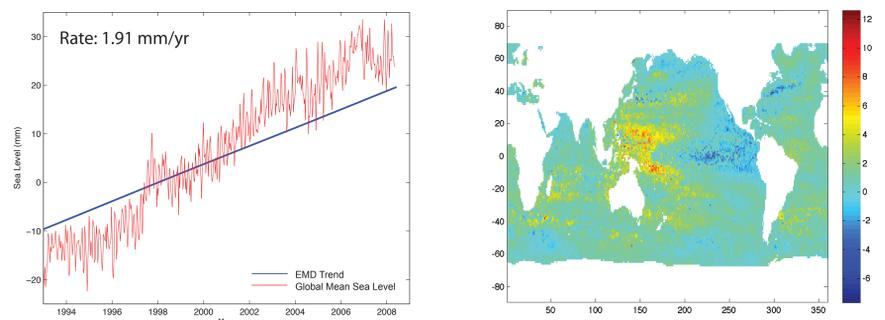
Figure 3. Global mean sea level rise time series and spatial map, as calculated from EMD and EOF analysis. As estimated from the time series, the rate of global sea level rise is estimated to be 1.91 mm/yr.
