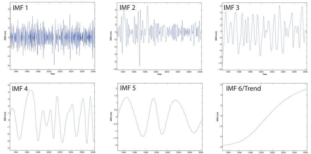
Figure 2. Empirical mode decomposition of sea surface height for a single 1x1 degree window over entire time series. The sum of the 6 IMFs will return the original data.
