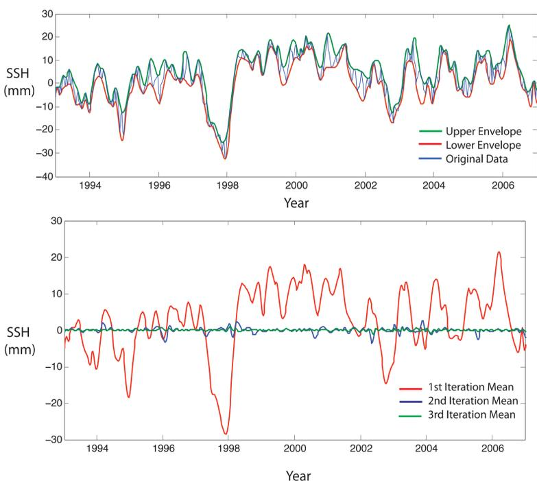
Figure 1. Top figure shows construction of upper and lower envelopes using cubic splines. Original data is shown in blue. Bottom figure shows mean of upper and lower envelopes calculated by successive iterations of the sifting process.
