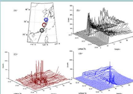
Fig.2 Series of 20Hz return waveforms of Jason1 cycle 164 track 229 across east mainland of China. (a) Black line indicates the ground track of 229. Three circles (black, red, blue) indicate the locations where waveforms in (b), (c), (d) are recorded, respectively. (b) A series of waveforms when Jason1 moved from ocean to land; (c) A series of waveforms when Jason1 is over land; (d) A series of waveforms when Jason1 moved from land to ocean.
