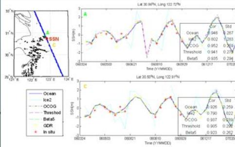
Fig.5 The time series of sea surface heights derived from Jason1 measurements using five retracking algorithms, and compared with in-situ measurements at tide gauge station SSN.
