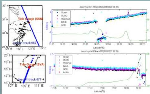
Fig.4 The sea surface heights derived from Jason1 measurements of track 062 (descending) and 077 (ascending) near tide gauge station SSN and SYA, respectively, using five retracking algorithms.
