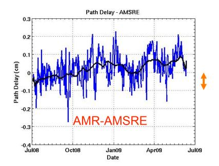
Comparisons between AMR and model and other radiometers
