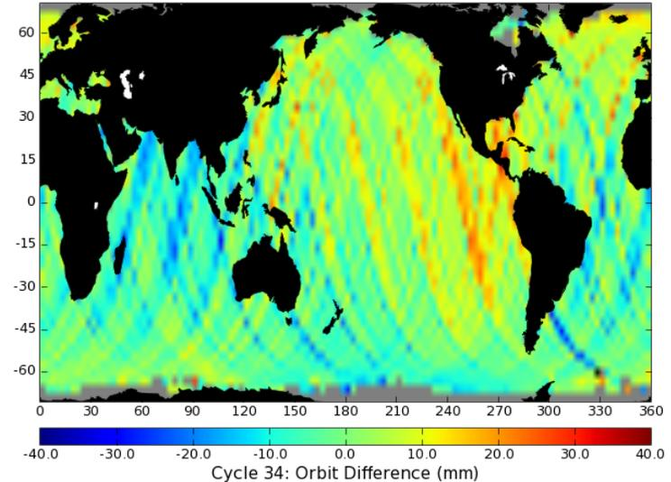
GPSOGDR orbit - GPS-based POE, (RMS, MIN, MAX) = ( 3, -14, 19 ) mm
