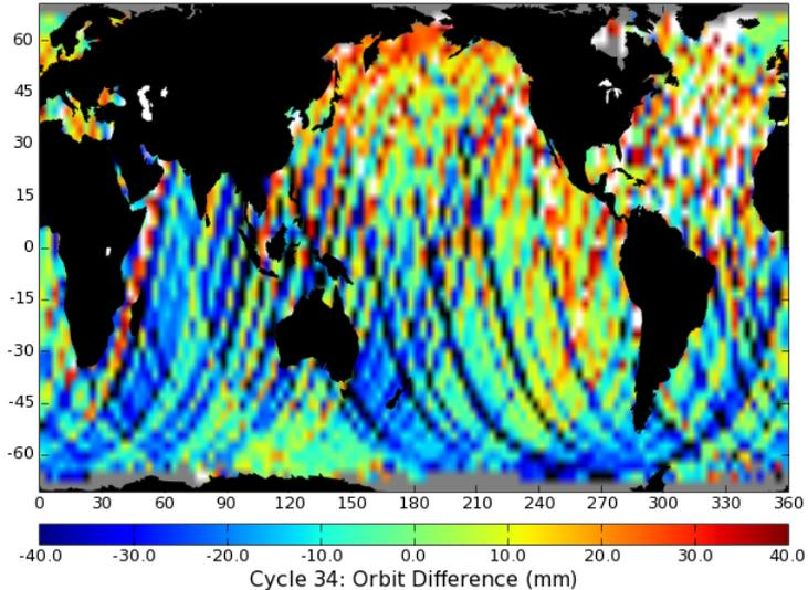
IGDR orbit - GPS-based POE, (RMS, MIN, MAX) = ( 9, -44, 44 ) mm
